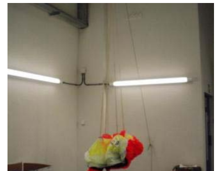
Fig. 2. Hang the canopy with the suspension lines at the same height. If the parachute is assembled on risers, make sure that they are the same length.
