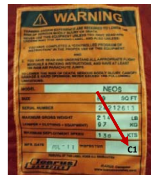
Fig. 17. When the modification is completed, mark "C1" with permanent marker in the inspector box on the warning label.
