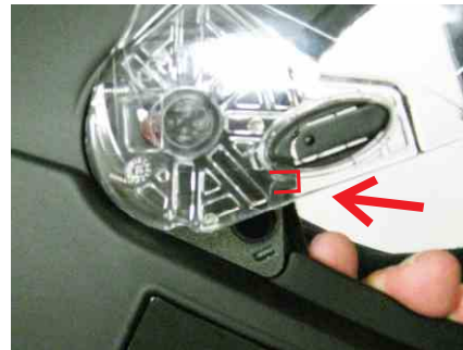
location of lens removal button as seen from outside
