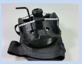
Step 4: Tighten the three screws until they're all gently snugged into place.
