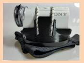
**Step 10:** Make sure the camera is fully seated in its socket. Some pressure may be required.
