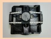
**Step 2:** Insert those screws into the three mounting holes.
