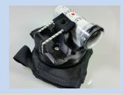
**Step 9:** Lift the other shock cord and continue sliding the camera in until it drops into place.
