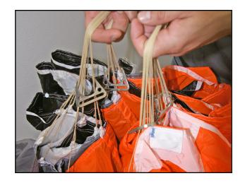
Clear the canopy lines as normal and bring the RDS rings towards the canopy as if a slider were attached.
