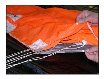
Two other snaps are located on the stabilizer perimeter tape, just aft of the C-line attachment points.
