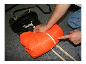
NOTE: It is critical to route the excess lanyard directly over the middle of the s-folded stack of canopy as it is placed in the d-bag.
