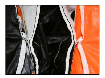
Fasten the trailing edge slider snaps onto the canopy's stabilizer aft edge's snaps.
