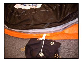
Then simply reattach the d-bag to the pilot chute attachment point on the top skin of the canopy, and the canopy can be deployed normally without the RDS. If desired, the slider can be removed upon deployment.
