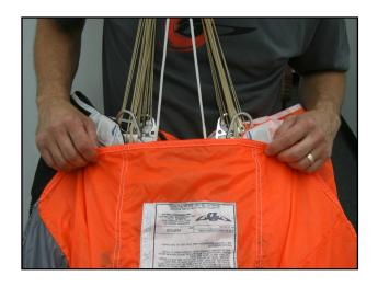
Run the lanyard and d-bag over the shoulder while completing the preparation of the canopy and wrapping up the tail during the pro pack.
