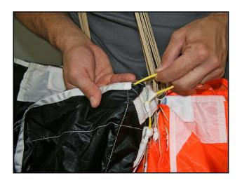
Fully stow the excess release cable along the edge of the slider into the pin sleeve as shown.
