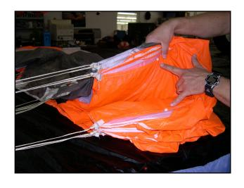
The Competition Velocity is equipped with plastic snaps that help secure the slider to the canopy during packing. Two snaps are located on the leading edge tape of the center cell.
