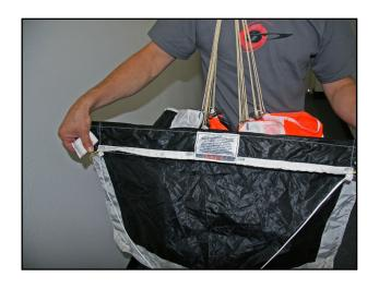
Orient the slider for ring attachment such that the warning label is readable. The white tape should be facing away with the lanyard coming off the trailing edge running freely towards the tail of the canopy.
