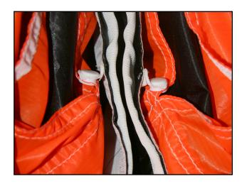
Fasten the leading edge slider snaps onto the canopy's leading edge center cell snaps.
