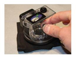
Rotate the housing to desired angle, then use the hex L-key to tighten another 1/8 - 1/4 turn
