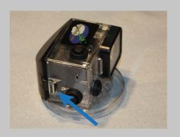
Insert three screws into the bottom of the housing
