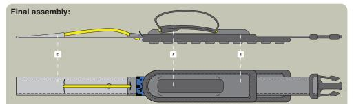
Now simply inset the loop on the end of the Cutaway Handle into the Comfort Strap's hole and put the Cutaway cable end inside the Webbing's pocket. This concludes the reassembly of your Cutaway Chinstrap. All you need to do now is to fit it in your helmet by using the provided hardware.
